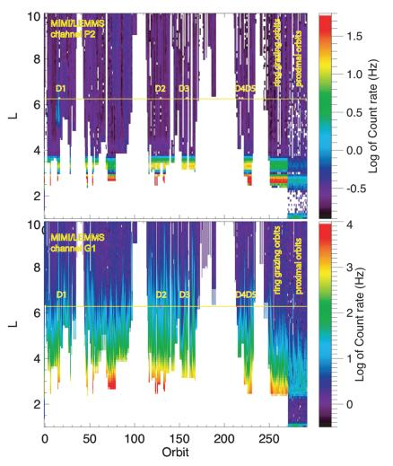
**Figure 1.** Color-coded count rates of protons (Channel P2 [2.3–4.5 MeV]) in the upper panel and electrons (Channel G1 [>1 MeV]) in the lower panel measured with MIMI/LEMMS for the entire Cassini mission as a function of orbit number (time) and L-shell. Dione's L-shell is shown with a yellow horizontal line. The times of the five Dione flybys are marked with D1 to D5.
