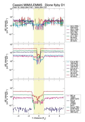
**Figure 6.** Cassini MIMI/LEMMS measurements of ions at various energies in Channels A0 to A4 (upper panel) and of electrons with keV to several MeV energies (middle and lower panels) during the D1 Dione flyby. While the C and BE channels measure electrons from the low-energy end of the sensor, the E-channels register electrons from the opposite side (high-energy end of the sensor). The yellow-marked region indicates the width of the moon.
