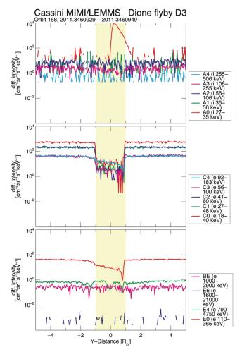
**Figure 8.** Cassini MIMI/LEMMS measurements of ions and electrons during the Dione Flyby D3. Same format as Figure 6. Please note that the differential intensity for Channel A0 in the upper panel is light-contaminated and not real.
