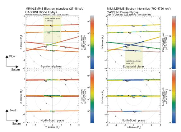
**Figure 4.** Color-coded electron intensities in MIMI/LEMMS Channels C1 (27–48 keV) on the left and E4 (790–4,750 keV) on the right during all five Dione flybys marked with D1 to D5 of the Cassini spacecraft. Dione is in the center of the coordinate system, and the spacecraft trajectories are projected into the equatorial plane (upper panels) and in the north-south plane perpendicular to the equatorial plane (lower panels).
